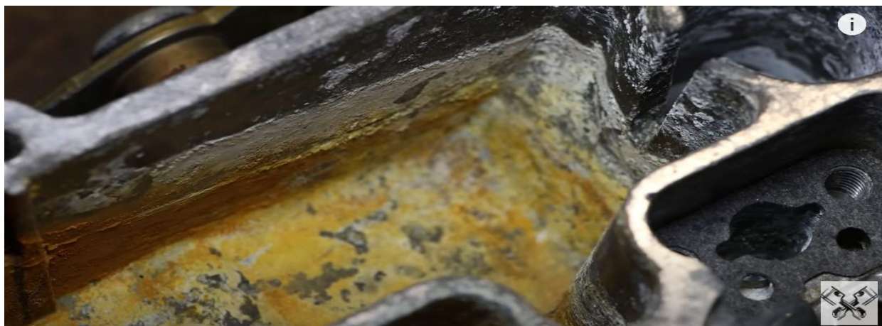
Corrosion of a carburettor caused by E10 fuel
